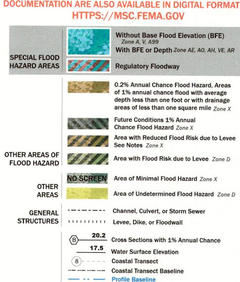
**Hydrographic Feature** Base Flood Elevation Line (BFE)
